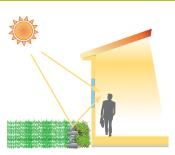
Visible transmittance (Tvw) measures how much light comes in through a window. It is an optical property that indicates the amount of visible light transmitted.
