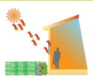
Solar Heat Gain Coefficient (SHGCw) measures how readily heat caused by sunlight flows through a window. The SHGCw is the fraction of incident solar radiation admitted through a window, both directly transmitted, and absorbed and subsequently released inward.
